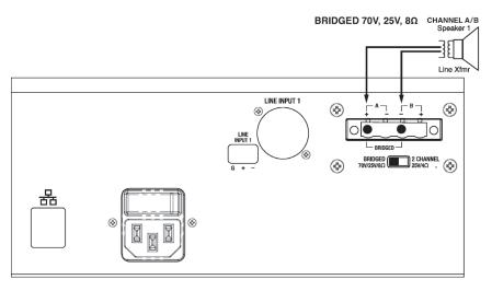
Figure 1. Bridged Wiring Diagram
