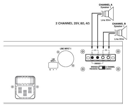
Figure 2. Two-Channel Wiring
