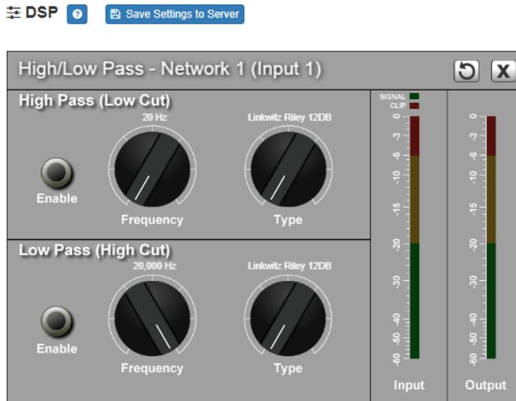
**Figure 11, High/Low Pass Parameters**
