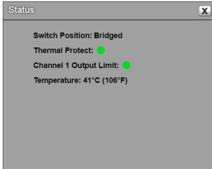
**Figure 21, Status for Bridged Channel**
