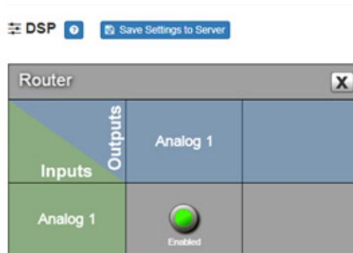
**Figure 16, Router for Single Channel Bridged Mode**
