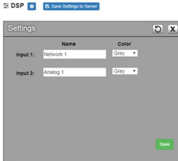
**Figure 18, Settings Parameters for Single Channel Bridged**
