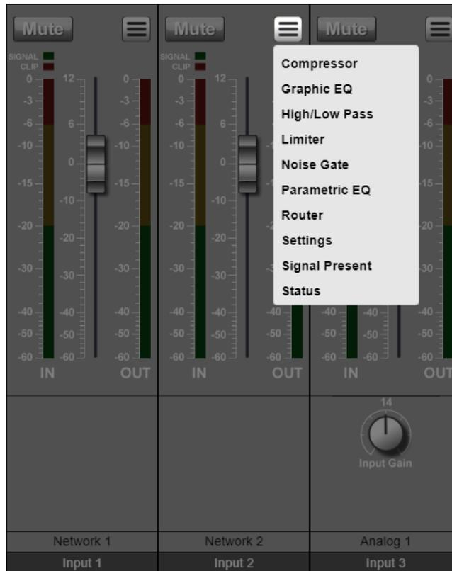
**Figure 7, DSP Page with Channel Drop-Down Menu**
