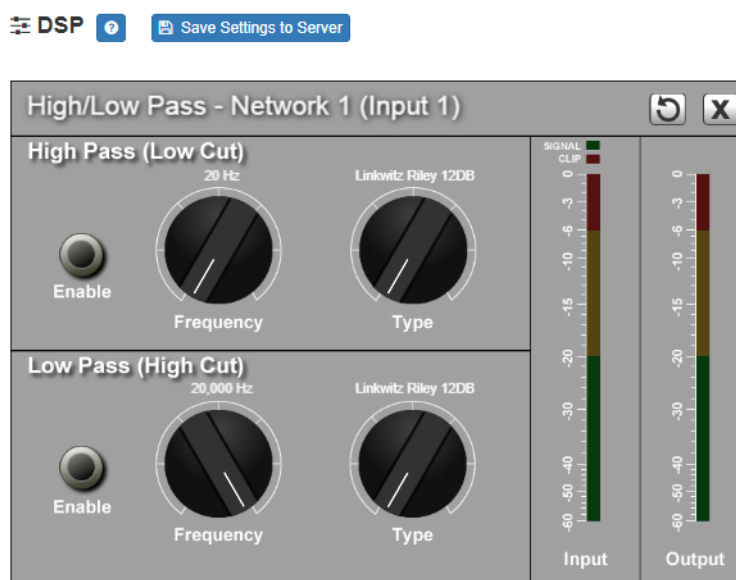
Figure 10, High/Low Pass Parameters
