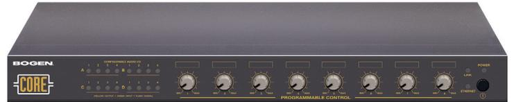
The Bogen CORE is a highly versatile digital mixer/processor designed for small to medium installations. Flexible hardware configurations, in blocks of 4: for 4 in/12 out, 8 in/8 out, etc. The CORE's PC-based software allows for design, downloading, reversal of in-box designs, and live monitoring, calibration, and routing. Three system hardware configurations are available: CORE8X8 (8 inputs, 8 outputs), CORE4X12 (4 inputs, 12 outputs), and CORE12X4 (12 inputs, 4 outputs).
