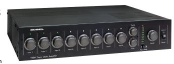
Each model includes eight module bays for input modules and allows up to four levels of priority between modules. Two module bays are also capable of accepting signal-processing output modules. Each input channel has an associated signal/clip LED for signal status. An 11-segment LED output meter monitors output signal level, which can be controlled by the Remote Volume Control Panel (RVCP, sold separately). Modules are required, but sold separately.
