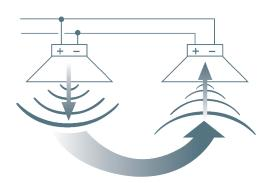
Reversed polarity in one speaker causes the sound between the speakers to be cancelled, mostly affecting the bass
