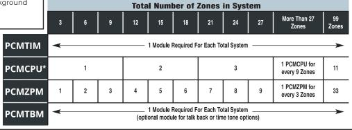
\*Note: One PCMPS2 Power Supply (not included) is required for each PCMCPU Module.
