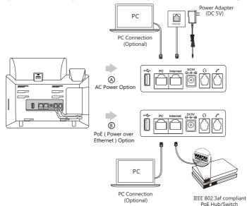
Note: The IP phone should be used with Yealink original power adapter (5V/2A) only. The use of the third-party power adapter may cause the damage to the phone. If you are connecting a PC to your phone, we recommend that you use the Ethernet cable provided by Yealink. If inline power (PoE) is provided, you don't need to connect the power adapter. Make sure the hub/switch is PoE-compliant.
