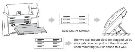
Note: You can also mount the phone to a wall. For more information on how to attach the wall mount bracket, refer to Yealink Wall Mount Quick Installation Guide for Yealink IP Phones.
