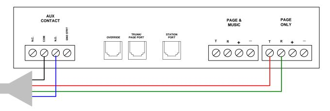
The DFT120 is designed to accept a Loop Start, Page Port, or a Page Port . If these are not available the UTI1 will be required.
