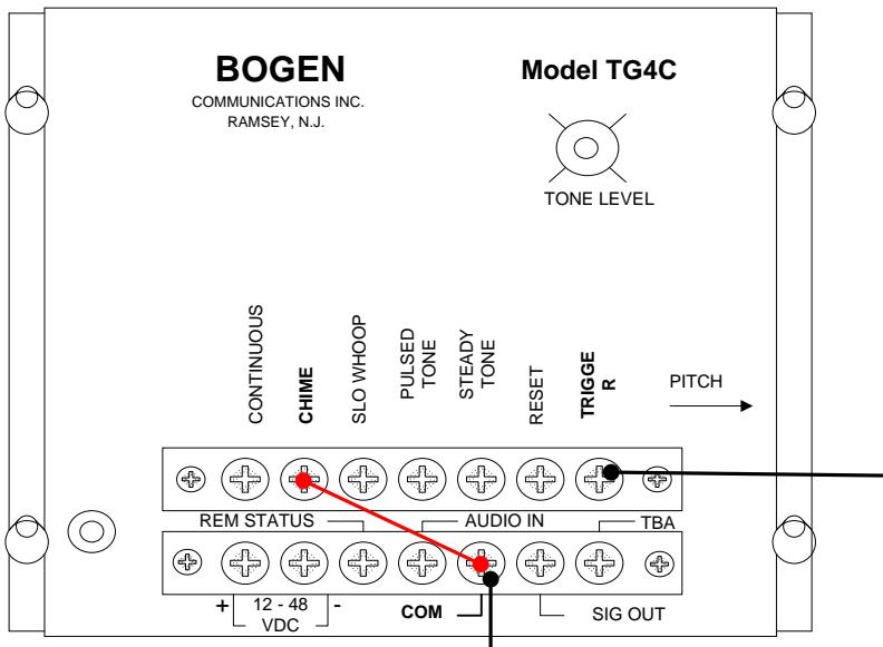
In this configuration the TG4C will sound for approx. 3 seconds when the Doorbell is pressed
