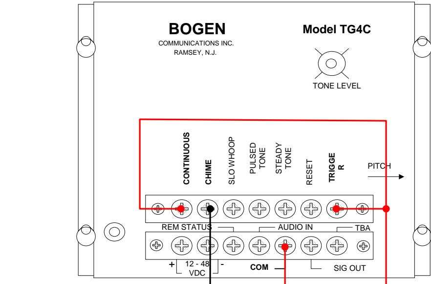
In this configuration the TG4C will sound for as long as the the Doorbell is pressed
