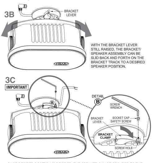
ONCE DESIRED POSITION IS DECIDED, THE SPEAKER CAN BE SECURED TO THE CLAMP. CLOSE THE BRACKET LEVER UNTIL FLUSH WITH BRACKET CLAMP. AS THIS IS DONE THE BRACKET BECOMES FIRMLY ATTACHED TO THE CLAMP. INSERT THE SUPPLIED SOCKET CAP SAFETY SCREW THROUGH THE HOLE IN THE END OF THE LEVER AND INTO THE BRACKET CLAMP. USING SUPPLIED WRENCH TIGHTEN SAFETY SCREW UNTIL IT IS IN CONTACT WITH THE BRACKET (DETAIL B). THIS PROVIDES A SECURE LOCK FOR THE BRACKET.
