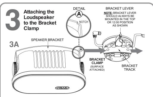
ONCE THE BRACKET CLAMP HAS BEEN SECURELY MOUNTED, THE BRACKET AND SPEAKER ASSEMBLY CAN BE ATTACHED. THE SPEAKER BRACKET HAS A "NOTCHED" END (SEE DETAIL A) THAT WILL BE FED FIRST, LEFT TO RIGHT, INTO THE BRACKET TRACK ON THE CLAMP. MAKING SURE THAT THE BRACKET LEVER IS UP, GENTLY SLIDE BRACKET/SPEAKER ASSEMBLY INTO THE TRACK.
