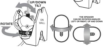
The Speaker can now be positioned in a variety of angles. To focus the speaker orientation in an upward or a downward manner, tilt the speaker in a back-and-forth motion within the Speaker Bracket Slot (D) amd Mount Bracket Thread (C) axis. The Speaker can also be rotated on an angle or side-to-side using the "Ball & Socket" design of the brackets and then locked into position by the Clamping Knob (see next section).
