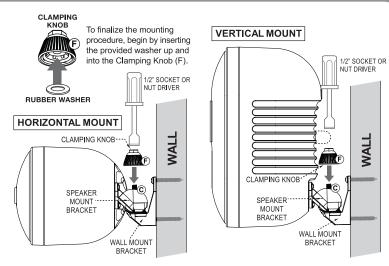
With the Speaker Assembly now in its final desired orientation, secure it into position by bringing the Clamping Knob (F) down on to the exposed portion of the Wall Mount Thread (C) and then screw the knob into place. A 1/2" Socket or Nut Driver can be used to firmly tighten the Clamping Knob so the entire assembly is now secured.
