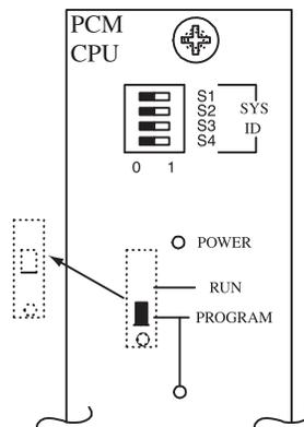
1. Remove the switch lock on the PCM CPU module and place the PROGRAM/RUN switch to the PROGRAM position (down). The green LED will illuminate.
