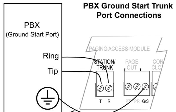
Wiring to the ground start trunk port requires a connection between the TAMB2's G/S terminal and the ground of the PBX. The AC chassis ground for the PBX can typically be used for this connection.
