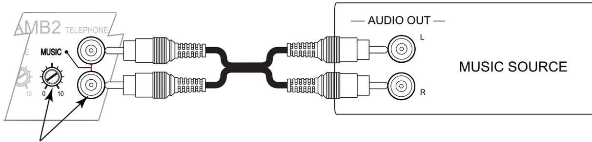
The TAMB2's Music Input will combine a stereo signal into mono or a mono source can be connected to either of the two RCA jacks. The MUSIC control is used to set the level of the music source when playing through the paging system. Set the level of the page using the amplifier's level control, then use the TAMB2 music control to set the background music level.
