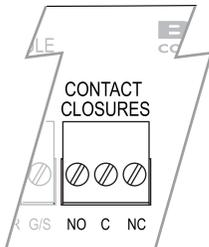
The contact closure contact set is provided to signal to external equipment the TAMB2's operational state. The contact set is single pole, double throw, and changes state from what is screened below the terminals when the TAMB2 becomes active and returns when the unit becomes idle again.
