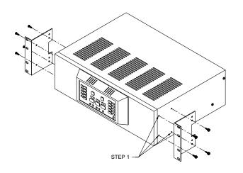
Step 1. Remove the 3 screws on each side of the PM3180 amplifier.
