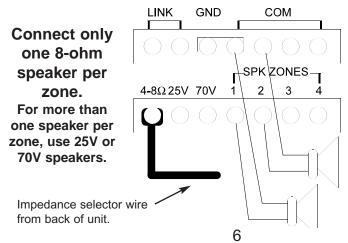
**To connect zones using 25V or 70V line:** Connect the impedance selector jumper to the 25V or 70V terminal. Connect the line to the desired zone terminal and COM as shown below.
