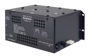
The Model MC2626B Power Supply is an unregulated, linear power supply providing nominal +26V and -26V @ 4.0A from 120V AC. Power consumption is 230W maximum.
