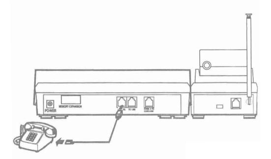
To verify the correct connection, pick up the handset on the local extension telephone. You should hear dial tone even if Cordless *Friday* is not powered.
