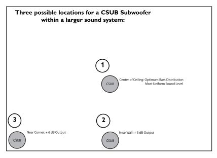
**Note:** The CSUB may be placed as close as 5" from a wall, provided care is taken to ensure that mounting clamps are properly extended (see *Installation* section). If mounting clamps cannot be properly extended, another location must be found.
