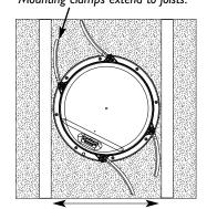
14-1/2 Inches between ceiling joists.
