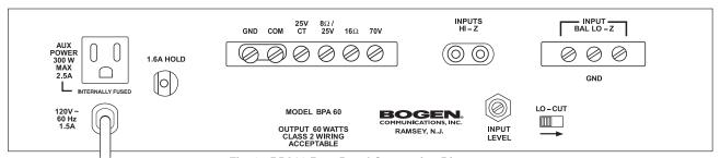
Fig. 1 - BPA60 Rear Panel Connection Diagram
