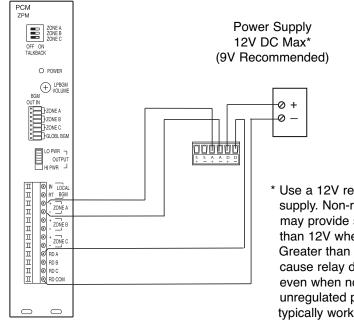
Use a 12V regulated power supply. Non-regulated supplies may provide significantly more than 12V when not fully loaded. Greater than 12V supply will cause relay driver to conduct even when not active. A 9V unregulated power supply will typically work appropriately.
