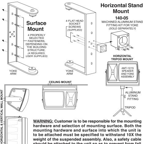
to be attached must be specified to withstand 10X the weight of the suspended assembly. Also, a safety cable should be attached to the unit so as to prevent from fall should the mounting hardware/surface attachment fail.
