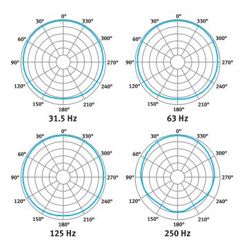
Horizontal and vertical measurements are identical.
