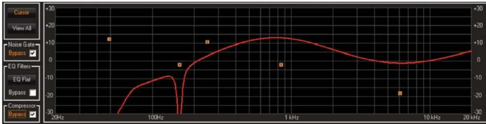
**Cursor:** The **InA/InB Editing** window also displays a graphic of the active EQ filters. By turning ON the “Cursor” feature, the Center Frequency and Gain can be adjusted by “dragging” the EQ cursor point with the mouse pointer.
