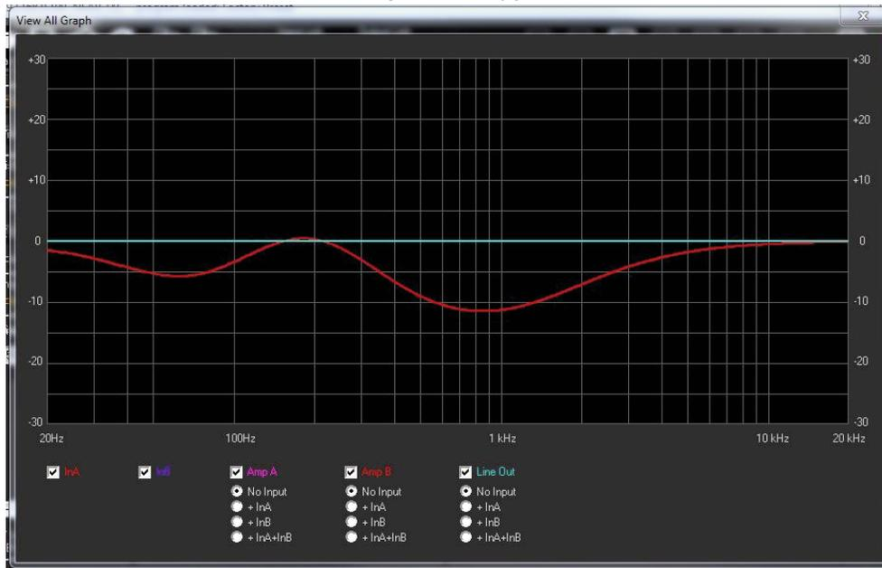
The **View All** window can be opened pressing the “View All” button. This allows the user to view all Input and Output response graphics. In addition, the Output response can be shown with and without the effects of Routed Input response.
