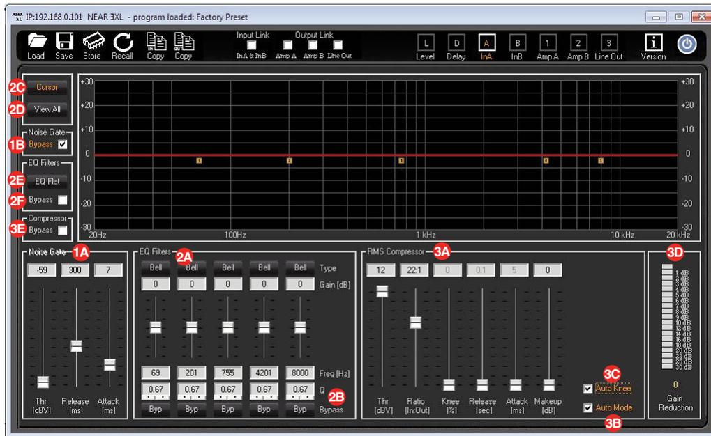
1. **Noise Gate:** Allows Noise Gate, when necessary, to improve the noise floor of an input source.
