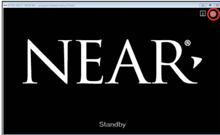
To Exit **Standby Mode**, press the red **On/Off Button** located in the upper right corner of the window. This will bring you directly to the **Home/Level** window.
