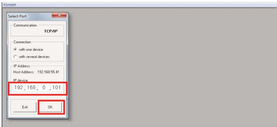
Enter the **Amplifier's IP Address (192.168.000.101 for the 3XL)** into the Select Port window and click **OK**; the GUI will then connect.
