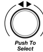
*NOTE: A Factory Restore can be accomplished by pushing and holding-in the Encoder/Push Button while simultaneously pressing the Power Switch ON. This will clear all user settings/presets and restore the unit to its factory defaults.*
