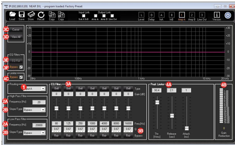
1. **Routing:** Matrix Input source selection for specific Output channel. Can be InA, InB, or InA+InB.
