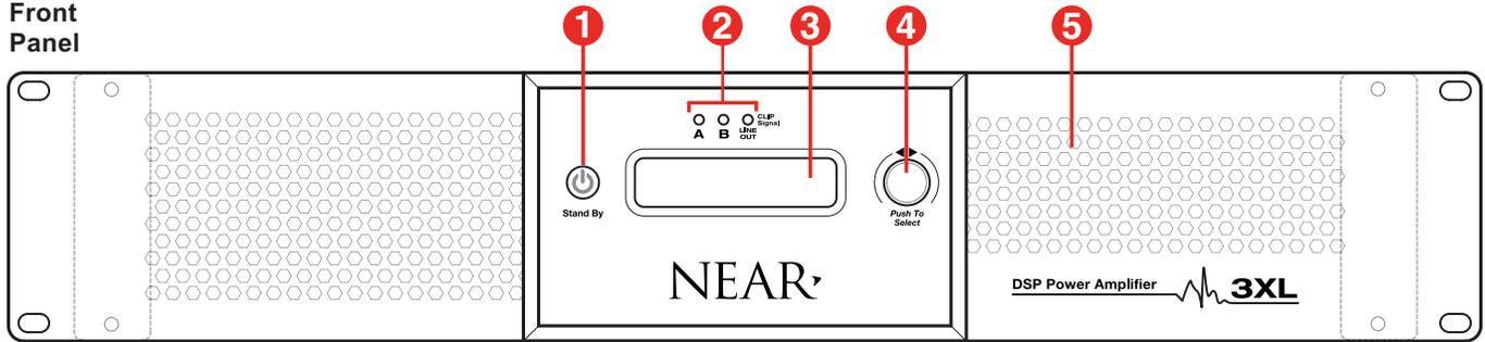
1. **“Stand By” Button** - Puts the amplifier into low-power consumption, or “Stand By” mode. The button will appear as back-lit Red when in “Stand By” mode.
