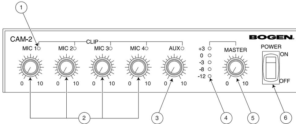
1. **Input Over Voltage LEDs (Clipping LED)** - LED will light when input is overdriven.
