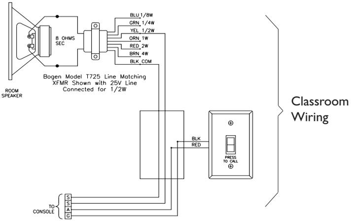
Figure 1 - CA15C Connecting Diagram
