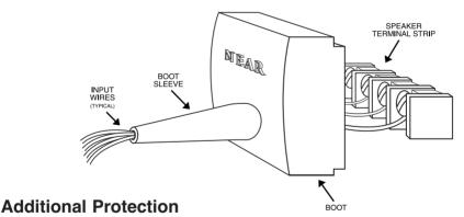
The terminal boot does not provide a water tight seal for the terminal strip. It is only designed to minimize the direct effects of weather on the wires and connections.
